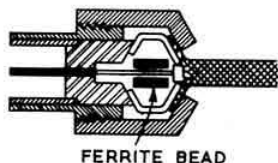
Fig. 5. G3HWR's co-axial sockets are made lossy to r.f. by means of a ferrite bead in order to stop r.f. from getting into a.f. circuits.
