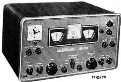
HQ170. Triple Conversion, selectable sidebands, full bandspread 6, 10, 15, 20, 40, 80 and 160 m. 17 tubes 100 kc crystal calibrator. Excellent performance, £184. (Other models in stock).
