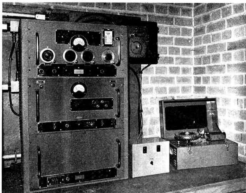
The equipment at GB3VHF. The transmitter rack is on the left of picture with the automatic keyer on the extreme right. The Venner time switch is mounted on the wall on the right of the transmitter cabinet.
